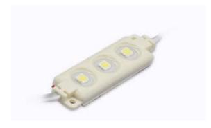
Designed for channel letter illumination in signage applications, the PAM6719 module provides bright and even illumination. Supplied in pre-wired chains of 20 pcs with 47mm link wires. Fixing is facilitated by a 3.0mm hole and 3M adhesive tape.
